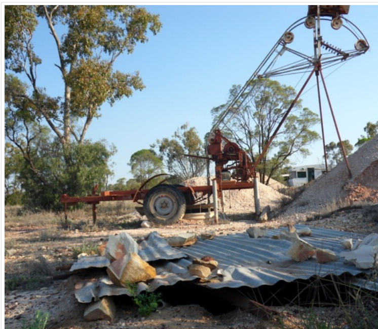
Mine shaft in foreground with rusty tin sheets and an extractor positioned over another mine s
